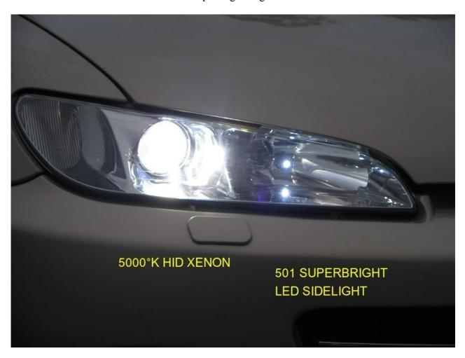
Adjust light unit to original position with no fixings tight. Face car towards a wall, adjust and tighten top fixings so that the horizontal cut-off beam on each light is the same level. Tighten remaining fixings and re-check beam pattern.
