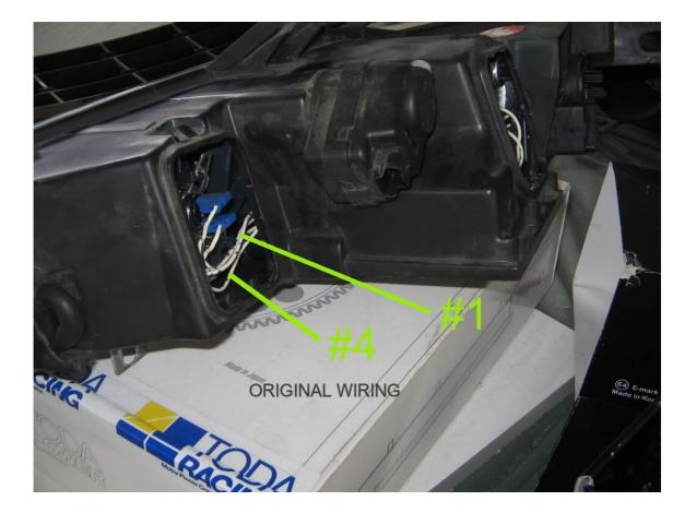
The wiring is almost foolproof as there are 3 different types of male/female connectors that will only fit together one way.
